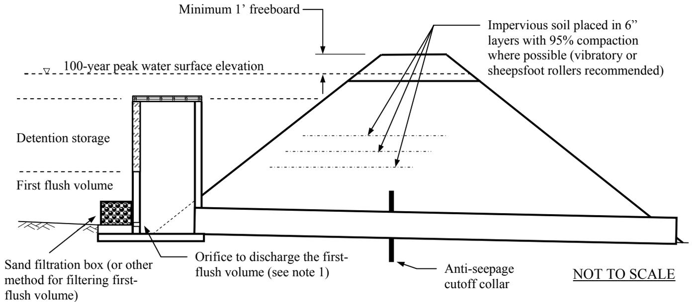
Typical Outlet Structure (V-notch)
